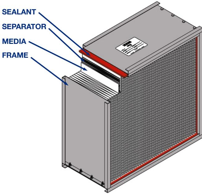
TRI-PURE™ HEPA HT and HEPAMAX™ HT filters use a stainless steel frame that is bolted together for added strength and rigidity required for demanding environments where high temperature filters are utilized.
