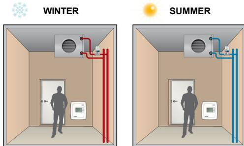
In 4-pipe installations, there are two separate pipe systems for heating and cooling with separate valves. The controller uses two outputs for control of heating and cooling in sequence.
